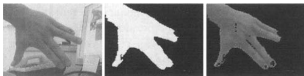
Figure 3: The image on the left is colour-segmented to find the skin-colour pixels (middle). The two images are then combined to produce the VideoArms image on the right.
