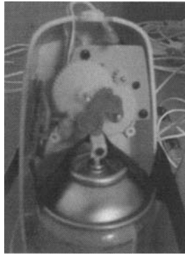
Figure 2: A built-in cam mechanism depresses the button of the aerosol as a toothed wheel rotates.
